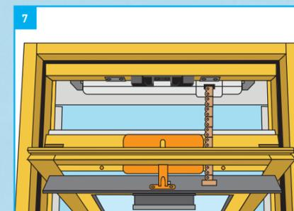
In order to attach the sash to the motor, fully extend the chain connector by pressing the down-arrow button on the wall mounted switch (fig 7). If you have opted not to fit a wall mounted switch you will then have to activate it using your remote control.
