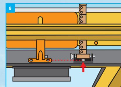
Once the chain is fully extended, use the connector bar to attach the chain to the vent flap bracket. Ensuring that you keep the chain straight, line up the vent flap bracket as shown (fig 8) and mark.
