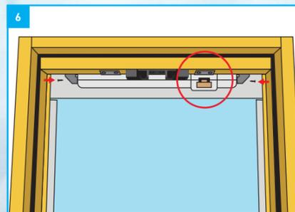
Fix the motor using 2 No. shoulder bolts. Ensure that the chain connector is facing inwards to the right of the latch keep (circled in fig 6). Once the motor is securely in position, feed the excess cable back up through the top of the frame.
