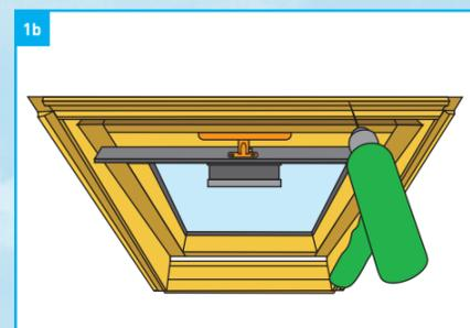
If the ceiling is finished a 10mm hole must be drilled through the top of the frame (figs 1b, 1c & 1d), 20mm down from top and 145mm in from the side of the frame.
