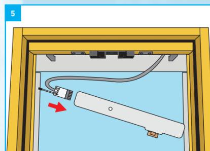
Plug the cable into the motor, ensuring that it is fully connected (fig 5).
