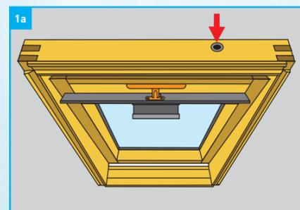
If the interior ceiling is not finished, the cable can be passed through the pre-drilled hole by removing the thimble (fig 1a).
