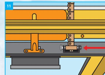
Feed the connector bar through the vent flap bracket and the chain connector. Secure with the cotter pin (fig 11).
